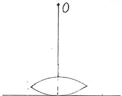
13-5. An object is placed a distance of 5cm from a thin convergent lens whose focal length is 10cm. Locate the image. (i) Is the image real or virtual? (ii) What is the magnification?
